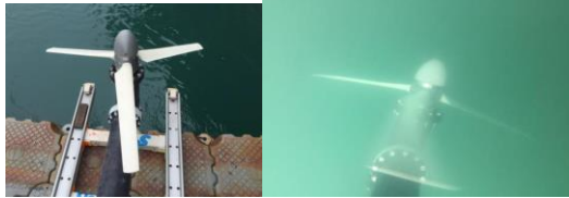
Figure 1. Scaled tidal turbine under field test.
