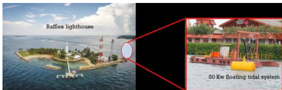
Figure 2. Deployment of floating tidal energy system in Singapore Waters.
