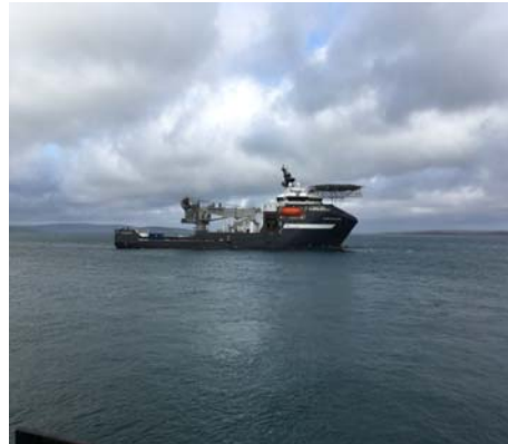
Figure 2: Larger DP vessel being used for a tidal turbine installation
